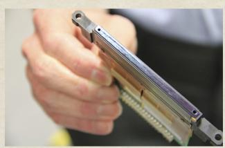
One key factor in achieving colour consistency is to properly maintain the printheads, to make sure that the nozzles are clean and fully operational.
